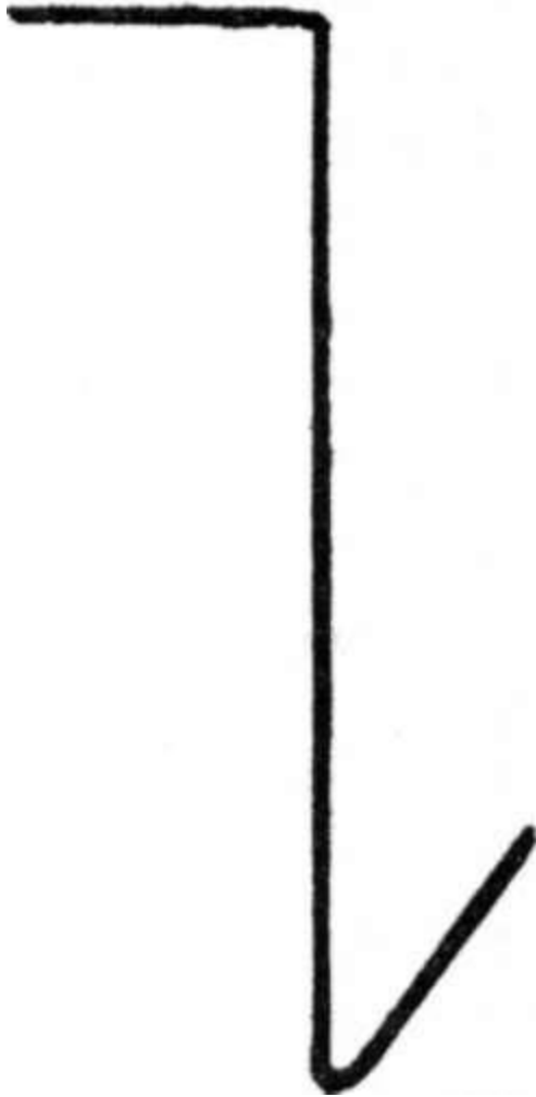
Figure 3. Dip wire - the first instrument.
